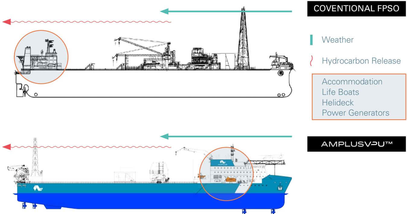
The ability to maintain a heading is also a benefit during shuttle tanker offloading operations and mitigate against the risk of fish tailing.
